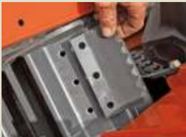
Optional set of intake combs for slippery or tall maize (standard on MC 180 S QUATTRO)
