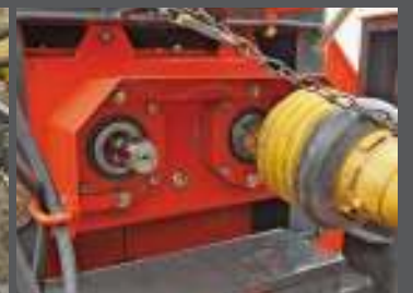
Two drive shafts for front and rear mounting
