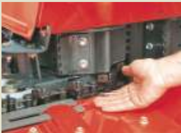
Extra shear bolt protection for the intake chain (MC 90 S TWIN and MC 180 S QUATTRO)
