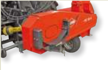
Trailer hitch in low position (MC 90 S and MC 90 S TWIN)
