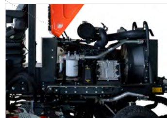
50.2 HP (37.4 kW) diesel Kubota® engine
