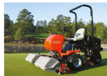
Walk through operator station
