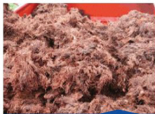
EFB placed into the bin and chopped for 10 mins
