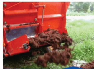
Hydraulically driven and controlled discharge chain conveyor
