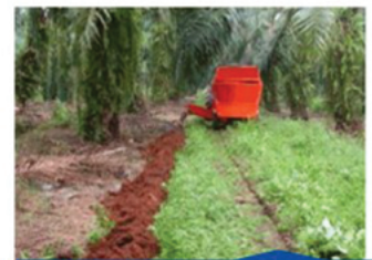
Discharge into palm path at rate of 10-12 tons per hectare
