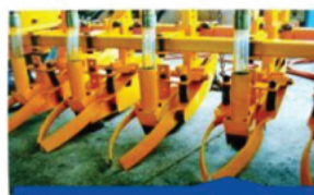
5 row sowing and row width is adjustable
