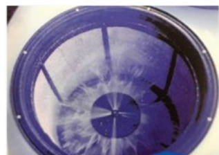
Automatic mixer on tank basket for powdered product
