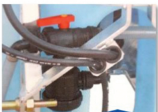
Suction filter with shut-off valve
