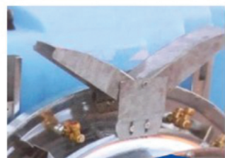
Directional wings to adjust spraying angle
