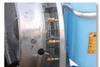
Gearbox lever to stop the fan
